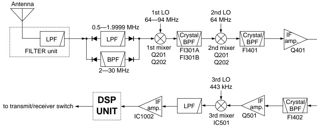
The IF amplifier (Q203) and resonator circuits are designed between the filter pair. The PLL output signal (1LO) enters the MAIN unit via the J601 and is amplified at the 1st LO amplifier (Q601). The amplified signal is passed through the 100 MHz cut-off low-pass filter (L604, L605, C604, C606-C610) to suppress harmonics components, and then applied to the 1st mixer circuit (Q201, Q202).
