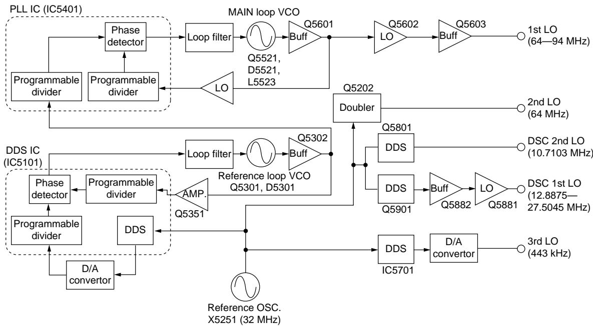
The detected signal output from the PLL IC (pin 2) is converted into a DC voltage (lock voltage) at the loop filter and then fed back to one of the VCO circuits (Q5521, D5521, L5523).
